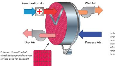
In the 1950s, Munters invented modern industrial dehumidification when it introduced the self-regenerating desiccant rotor, the heart of the dehumidifier.
